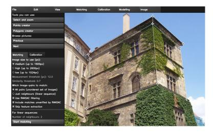
You don't have to mark the polygon on every photo where its vertices are visible. It suffices to do it once. Note that the vertices of a polygon are connected by lines even when some of them are not visible on the current photo. This might be a little confusing sometimes, if you have an idea how to better visualize this (you'll probably run into such situation at some point), write it on our wiki (it's on the project's website).
