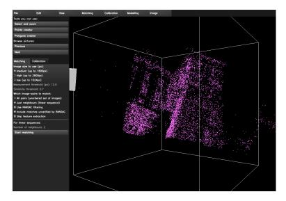
Sometimes, the point cloud seems deformed or just looks like random noise. That might be because there's a lot of mismatched tracks. The cameras still might be correctly calibrated, though. Use the Modelling > Triangulate, only trusted command to triangulate only the vertices that have a very high probability of being correctly tracked.
