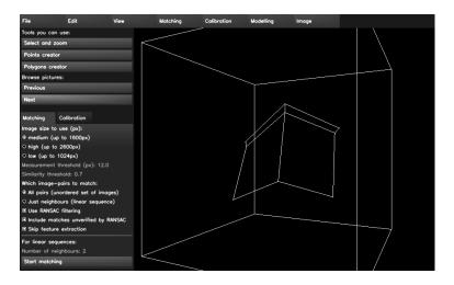
If some of the polygons are missing, it's probably because one or more vertices couldn't be correctly triangulated because they are marked inaccurately. Fix this by going back to Shot mode and correcting the points (since their position couldn't be trianguated, they do not have a green dot near them).
